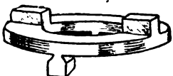
The brass "safety valve" coupling on the valve spindle with undercut tongues.
